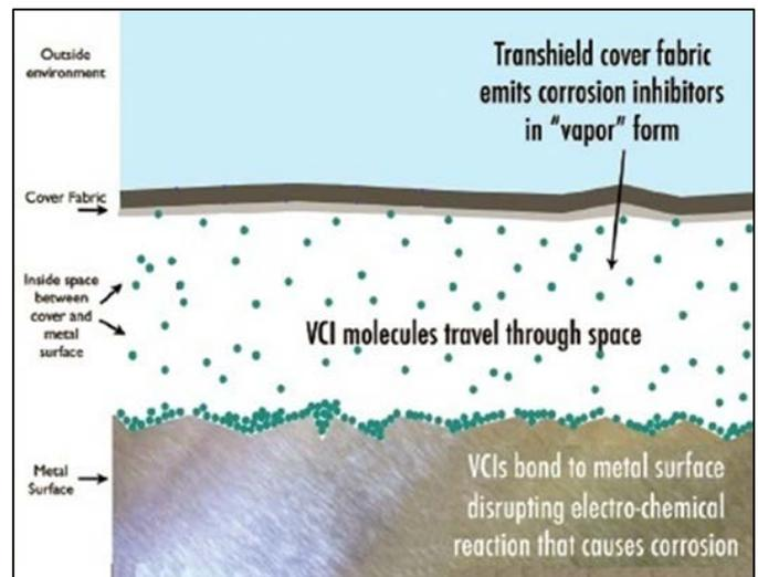
Figure 2. VCI in vapor form migrating and bonding to the metal.
