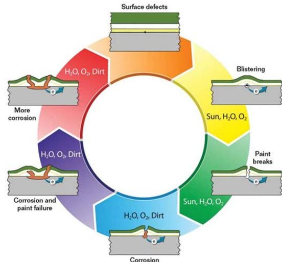
Figure 2. Paint failure and corrosion cycle.
